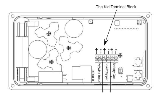
Rear View of The Kid with the back cover removed.
