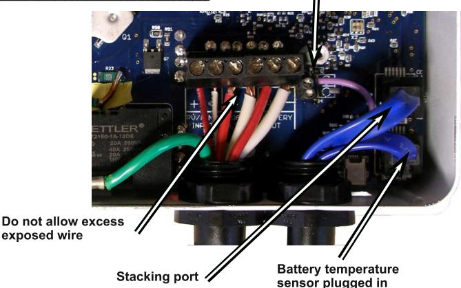
**Sample wiring** showing PV, Load/Clipper, Battery, Whizbang Jr., BTS and stacking cable. Wires may exit through either conduit fitting.
